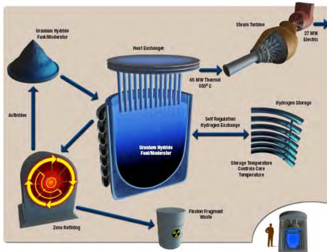
Figure 10-14 Simplified Hyperion Power Cycle Diagram (Source: Hyperion Power Generation)
