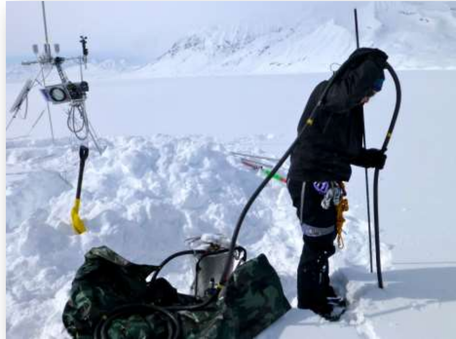
Installing an acoustic sensor for measuring/monitoring snow/ice surface change on West Fork Glacier (ESR1), Spring 2013.
