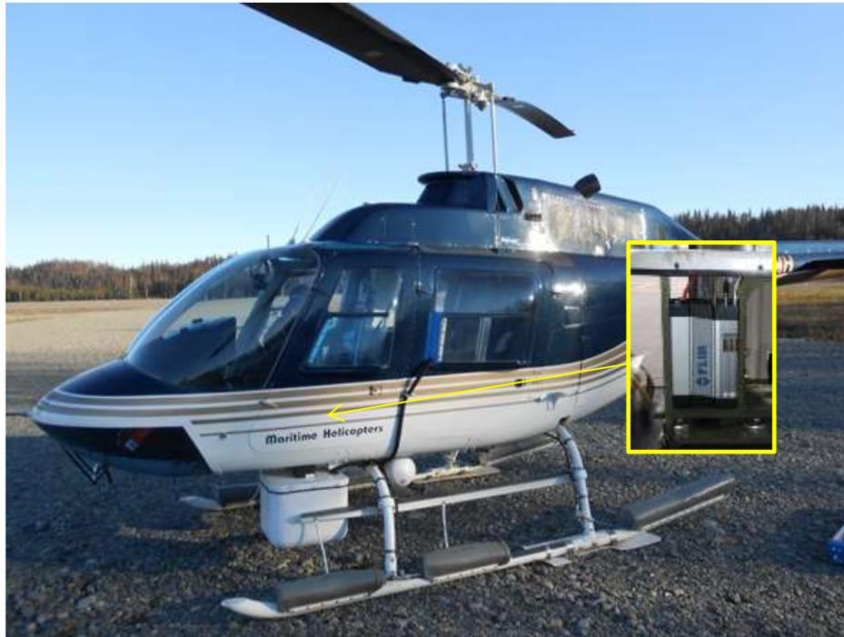
**Figure 2. Bell Jet Ranger equipped with mounted FLIR sensor.**
