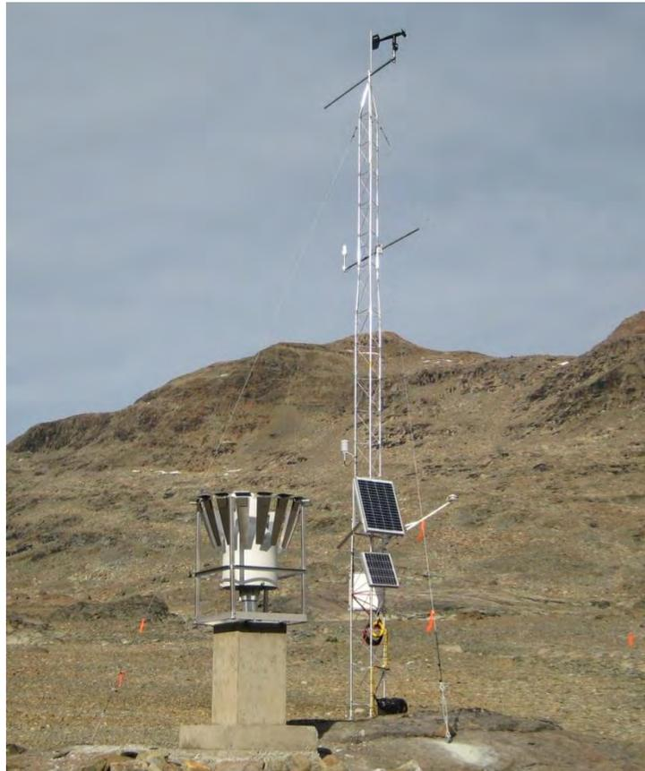
**Figure 3. Example Meteorological Station Installation**
